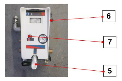
Delivery can be stopped at any time by using the flow stop button (7). To restart delivery press delivery start lever (5) and the remaining amount of water will be dispensed.
