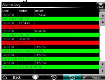
Figure 39: Alarms Log submenu.
