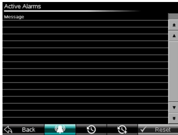
Figure 37: Active Alarms submenu.
