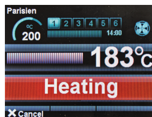
The heating screen shows the temperature progress.
