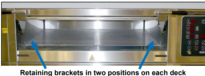
Figure 3: Installing the tile retaining brackets
