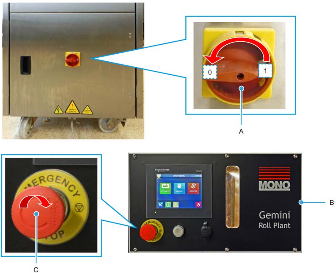
Figure 6.1: Emergency stop buttons
