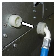
OVEN WATER CONNECTION AT REAR
